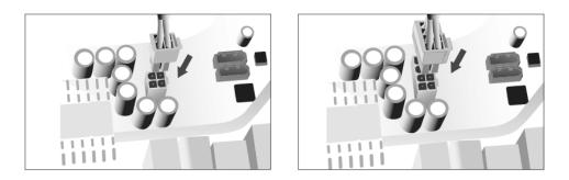
5. Connect extra cables from the cable pack to the sockets on the power supply only if needed. If you are going to plug the PCI-E cables into the PSU, they should go into the red sockets. If the red sockets are not being used for PCI-E, then they can be used for any other type of cable supplied in the pack that accompanies the PSU.
